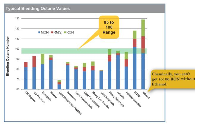
Very few refinery components exceed 95 RON – limiting the capability of refiners to improve pool octane to that level
